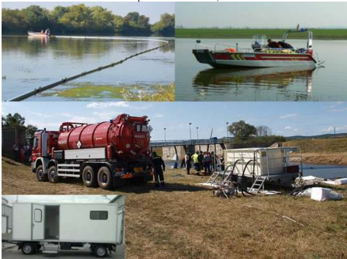
Picture No 2 Part of basic technical equipment of the company Transpetrol, a. s. intended for liquidation of crude oil accidents on water surface (metal breast wall, fire-brigade boat, ADR boat, oil substances separator and a caravan)
